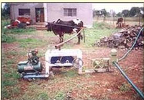
Animal driven Modern energy machine with air compressor & water pump
